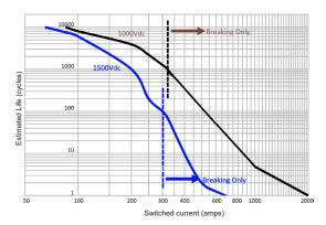
Fig 6: Typical estimated life graph with "Breaking only" indicated
