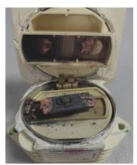
Fig 7: DEVR30 showing contact damage
