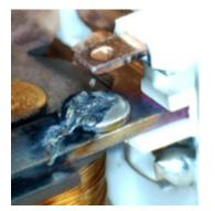
In the photo (left) can be seen what might happen if the magnet orientation is incorrect. In this example, the arc has been directed, by the magnet, up the contact blade instead of at 90' to the blade. The result is that the contact has melted because the arc was not extinguished quickly. This was after only 250 operations.
