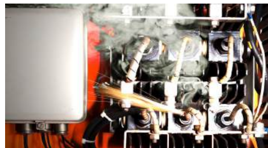
Contactor fire - no blowout magnet
