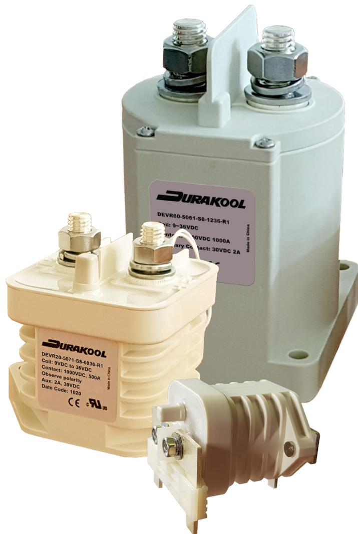
Typically, an electric vehicle (EV) will have two main contactors which are positioned in the feed from the battery to the electronic motor drive. There may be others used as part of the pre-charge, discharge or charging circuits. The principal function of the main contactors is to isolate the battery from the rest of the system when the vehicle is not being used and when an emergency occurs which requires immediate disconnection of the battery for safety reasons.
