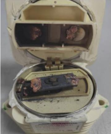
Fig 7: DEVR30 showing contact damage
