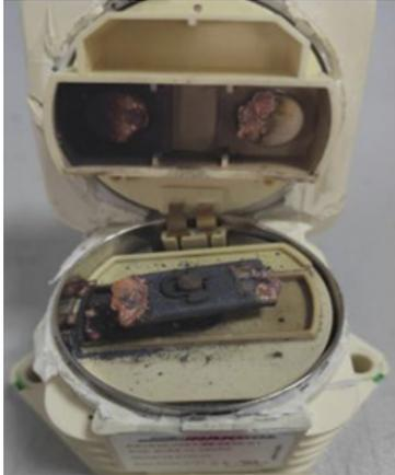
Fig 7: DEVR30 showing contact damage
