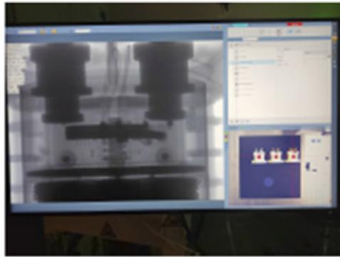
Fig 8: X-ray of DEVR30 showing contact damage
