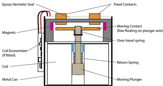
Fig 4: Typical epoxy seal design
