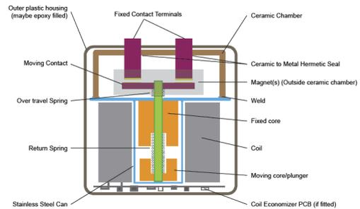
Fig 5: Typical ceramic chamber design
