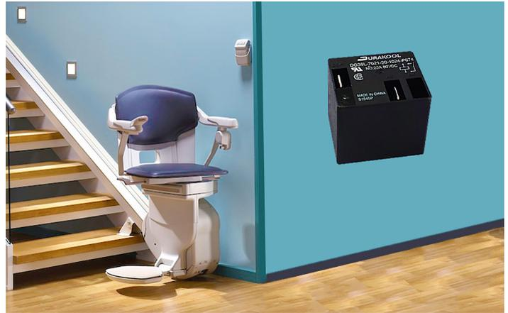
The DC motor control relay measures a compact 32.2 x 27.5 x 28mm and is designed to switch in applications where the DC voltage exceeds 24VDC. As the relay opens it will pull an arc. With other relays of this type, if the contact gap is not big enough, the arc will not go out until the relay is damaged. An internal magnet deflects the arc from the contact as the relay opens, thus extinguishing the arc.
