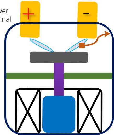
In the left drawing, you can see how the arcs are pushed away from the moving contacts.
