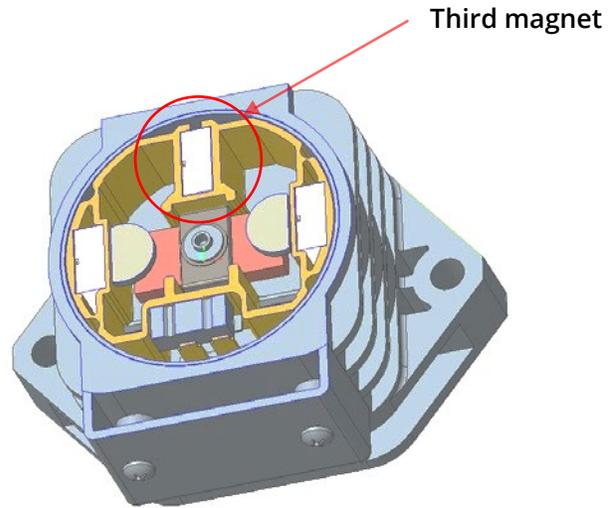
Non polarised contactors use a third magnet to move the arc away. This is why non polarised contactors are a little more expensive.
