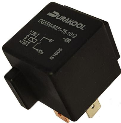
Pictured (left) is the Durakool DG55M relay. The magnet position can be seen on the side of the relay which can switch 80VDC, or more, at up to 20A in a standard Mini-ISO style automotive relay.
