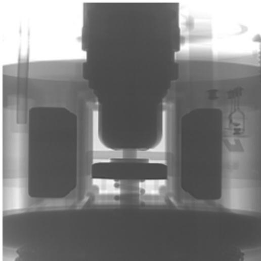
The X-ray photograph (left) shows an end on view of the contacts for the Durakool DEVR60 HVDC contactor. The magnets can be clearly seen either side of the moving contact bar. Comparison with the line drawing above makes it obvious
