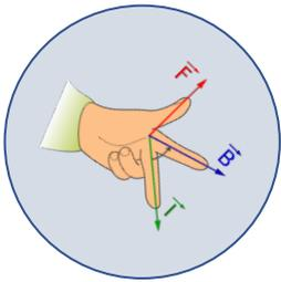
The switching arc is the conductor with a current flowing through it with the actual medium being the plasma between the opening contacts; and the magnetic field is applied from external magnet(s). These magnets are positioned to deflect the arc away from the opening contacts and, as a result, stretch the apparent contact gap to the point where the arc is no longer self-sustaining and goes out. In the diagram (left) the arcs are deflected outwards (F).
