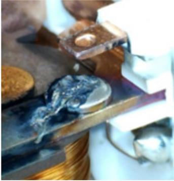
In the photo (left) can be seen what might happen if the magnet orientation is incorrect. In this example, the arc has been directed, by the magnet, up the contact blade instead of at 90° to the blade. The result is that the contact has melted because the arc was not extinguished quickly. This was after only 250 operations.
